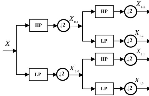
Fig. 1. Wavelet packet decomposition in two scales.
