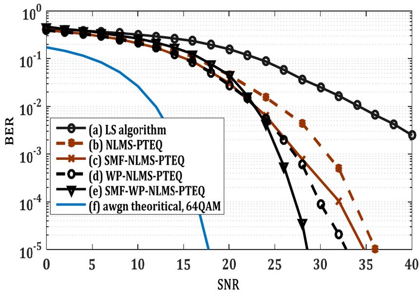
Fig. 5. Error performance curve, 64QAM signal, NLMS training and SMF-WP-NLMS-PTEQ under short CP
