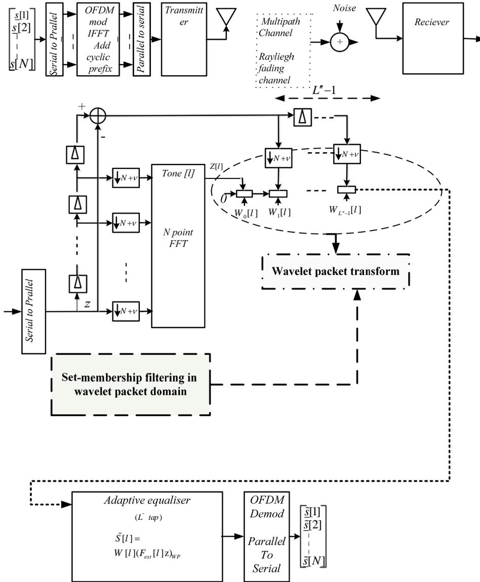
Fig. 3. SMF-WP-NLMS-PTEQ proposed algorithm block diagram
