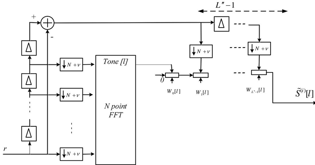
Fig. 2. PTEQ-OFDM receiver structure.
