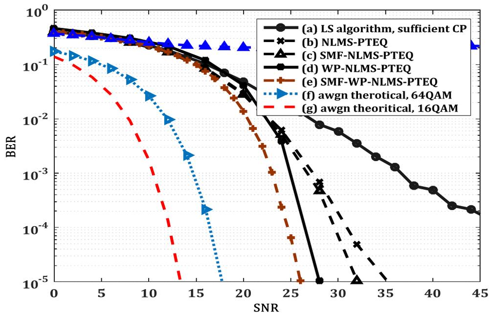
Fig. 4. Error performance curve, 16QAM signal, NLMS training and SMF-WP-NLMS-PTEQ under short CP
