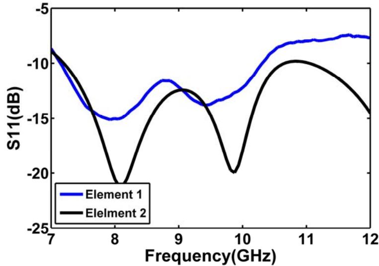
Fig. 3.  $S_{11}$  for different schemes of element 1 & element 2.
