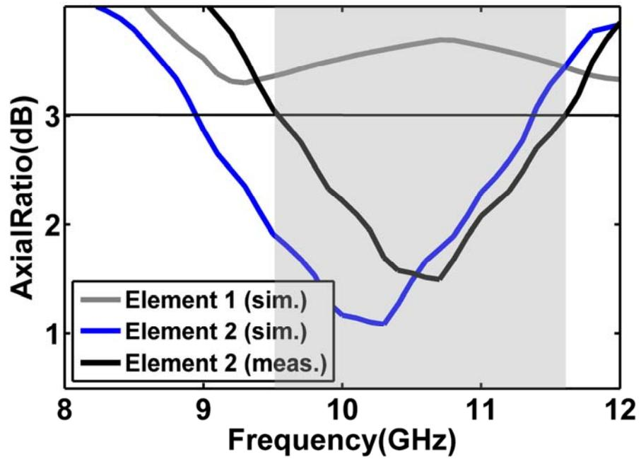
Fig. 6. Measured and simulated AR for RHCP X-Band Element1 and element 2.
