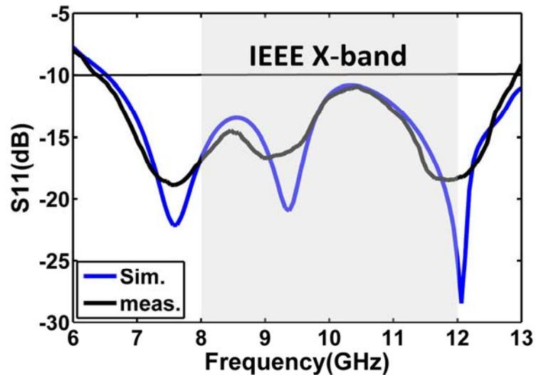
Fig. 4.  $S_{11}$  for RHCP wide-Band Element with parametric optimization.
