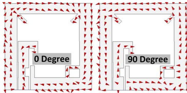
Fig. 5. Distribution of the surface current on the feed and ground of the structure at 10.5 GHz in  $0^\circ$  &  $90^\circ$  phases.
