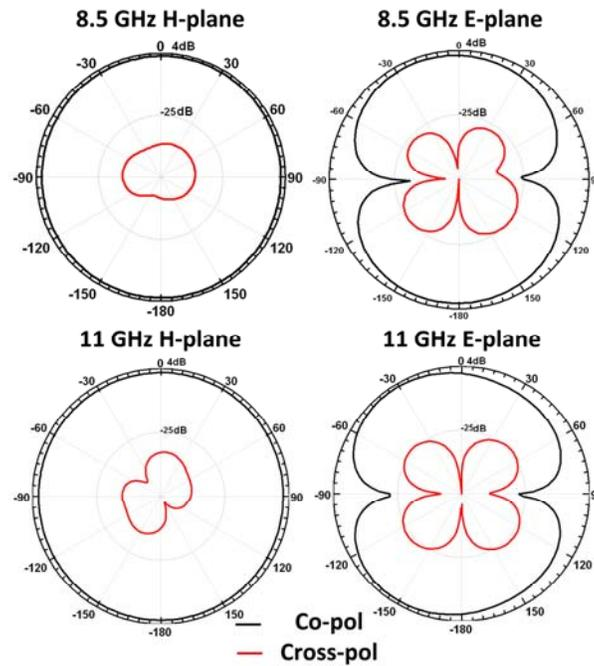
Fig. 8. Measured patterns of wide-band Element.
