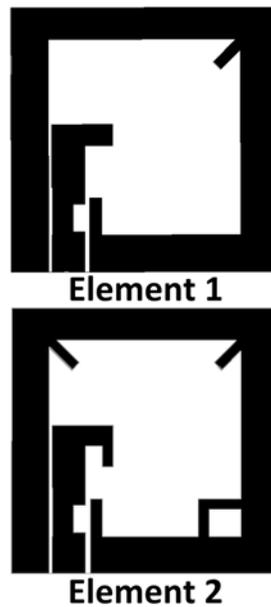
Fig. 1. Design process of ultimate RHCP X-band Elements.
