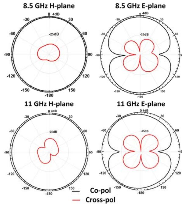
Fig. 8. Measured patterns of wide-band Element.
