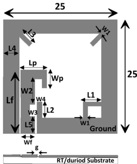
Fig. 2. Geometry of the proposed Asymmetrical-fed RHCP element.
