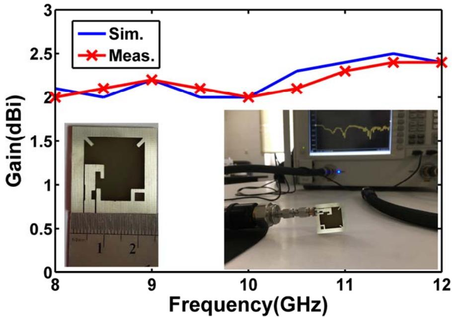
Fig. 7. Simulated and measured gain of RHCP X-band element 2.
