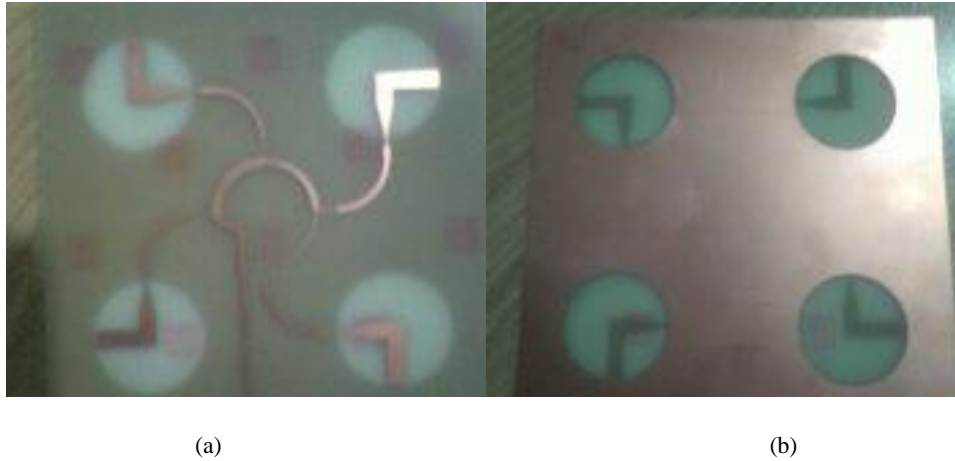
Figure 5. Photograph of the fabricated CPS antenna array, (a) front (b) behind.
