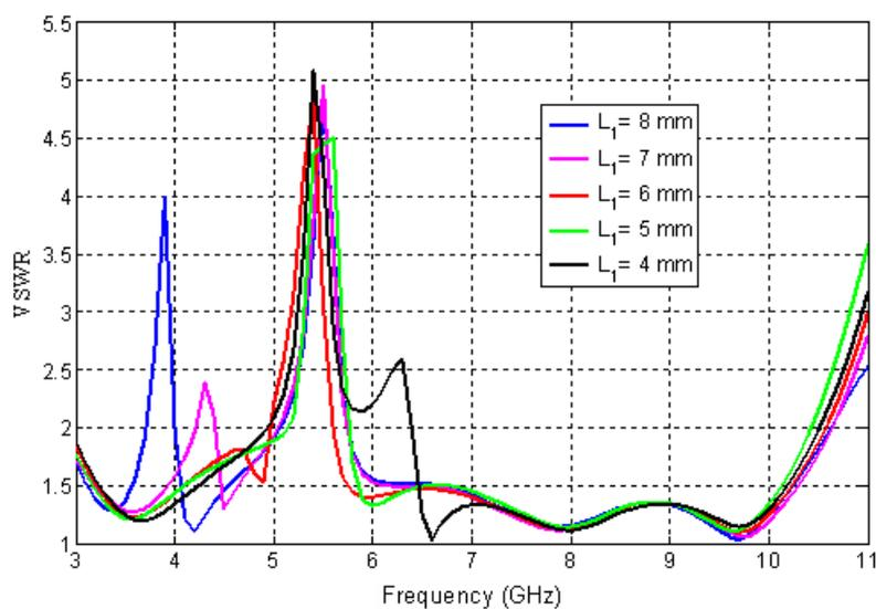
Fig. 3. Simulated VSWR of the proposed antenna for different values of  $L_1$
