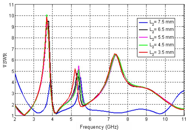
Fig. 4. Simulated VSWR of the proposed antenna for different values of  $L_2$
