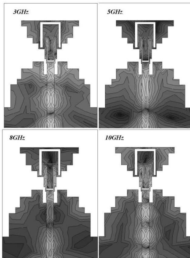
Fig. 6. Simulated current distributions for the proposed antenna at various frequencies
