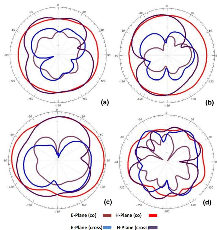
Fig. 7. measured radiation patterns of the proposed antenna(a) 3 GHz, (b) 6 GHz, (c) 8 GHz and (d) 10 GHz.
