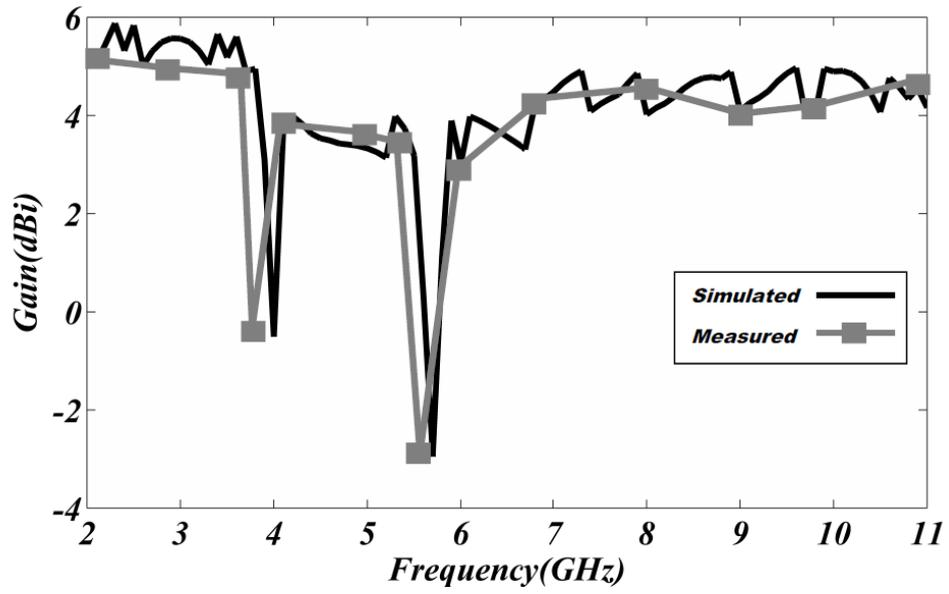
Fig. 5. Measured and Simulated gain of the proposed antenna
