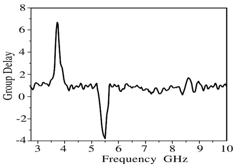
Fig. 8. Group delay of the proposed antenna
