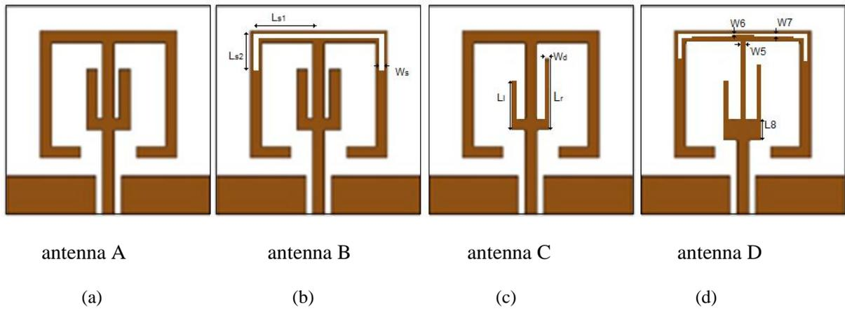
Fig. 2. Design evolution of the proposed antenna
