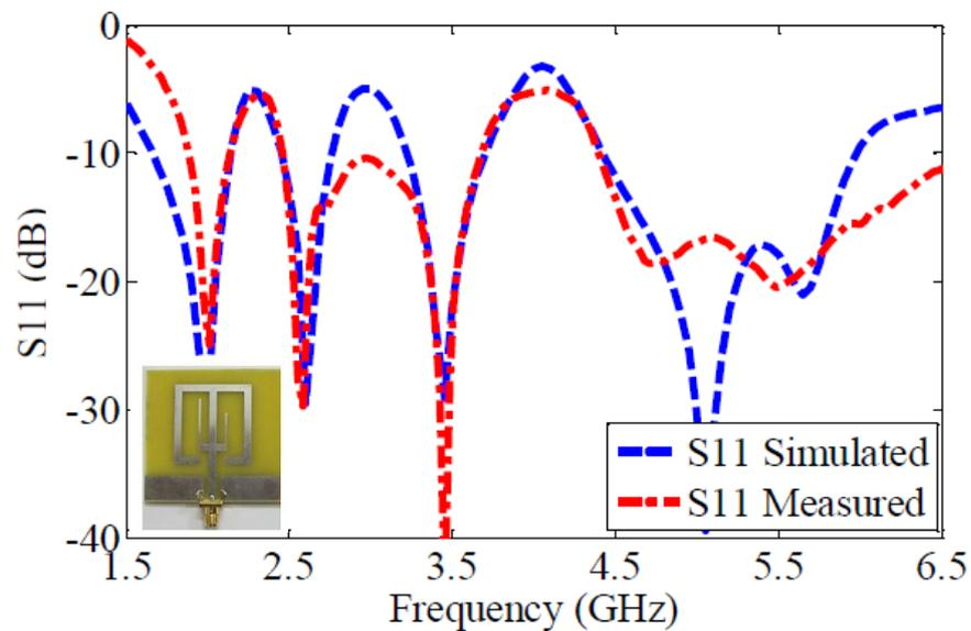
Fig. 10. Simulated and measured reflection coefficient of the antenna C shown in Fig. 2.
