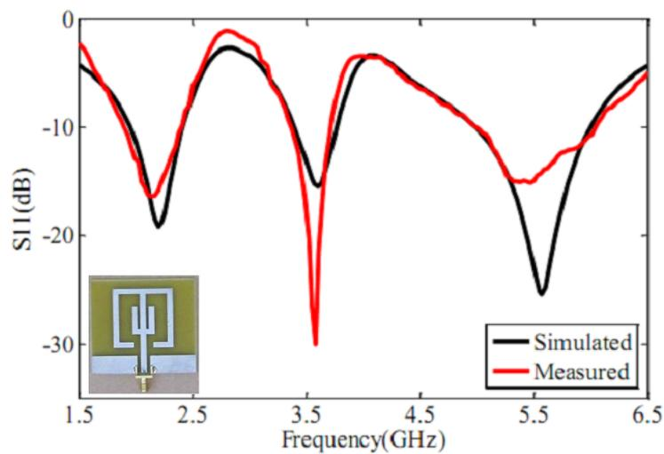
Fig. 4. The simulated and measured reflection coefficient of antenna A shown in Fig 2.
