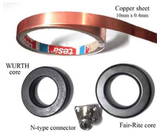
Fig. 3. Materials used in constructing the BCI-probe.
