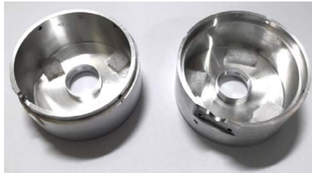
Fig. 18. The probe shield after cutting the most of its inner part.
