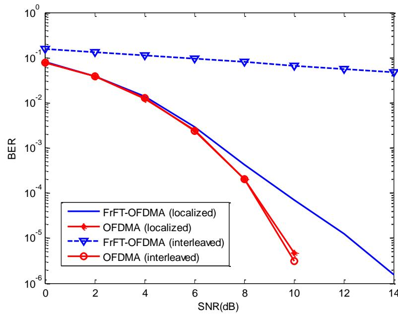
Fig. 4. Performance comparison of a 2-user OFDMA and non-orthogonal FrFT-OFDMA system in AWGN channel with different mapping schemes and  $M = 128$ ,  $\Delta T = 10^{-4}$ ,  $cota_1 = 636.62$  and  $cota_2 = 6.366 \times 10^4$ .
