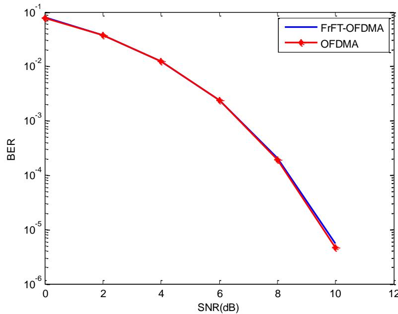
Fig. 3. Performance comparison of a 2-user OFDMA and quasi-orthogonal FrFT-OFDMA system in AWGN channel with  $M = 128$ ,  $\Delta T = 10^{-4}$ ,  $cota_1 = 0$  and  $cota_2 = 636.62$ .
