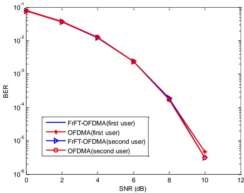
Fig. 5. Performance comparison of a 2-user OFDMA and non-orthogonal FrFT-OFDMA system in AWGN channel with spectral guard band and  $M = 128$ ,  $\Delta T = 10^{-4}$ ,  $cota_1 = 636.62$  and  $cota_2 = 6.366 \times 10^4$ .
