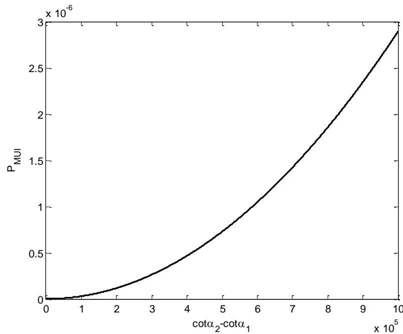
Fig. 1.  $P_{MUI}$  versus  $\cot\alpha_2 - \cot\alpha_1$  for an FrFT-OFDMA system with two users where  $M = 128$  and  $\Delta T = 10^{-6}$ .
