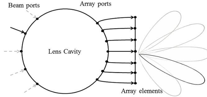
Fig. 1. Schematic of Rotman lens antenna
