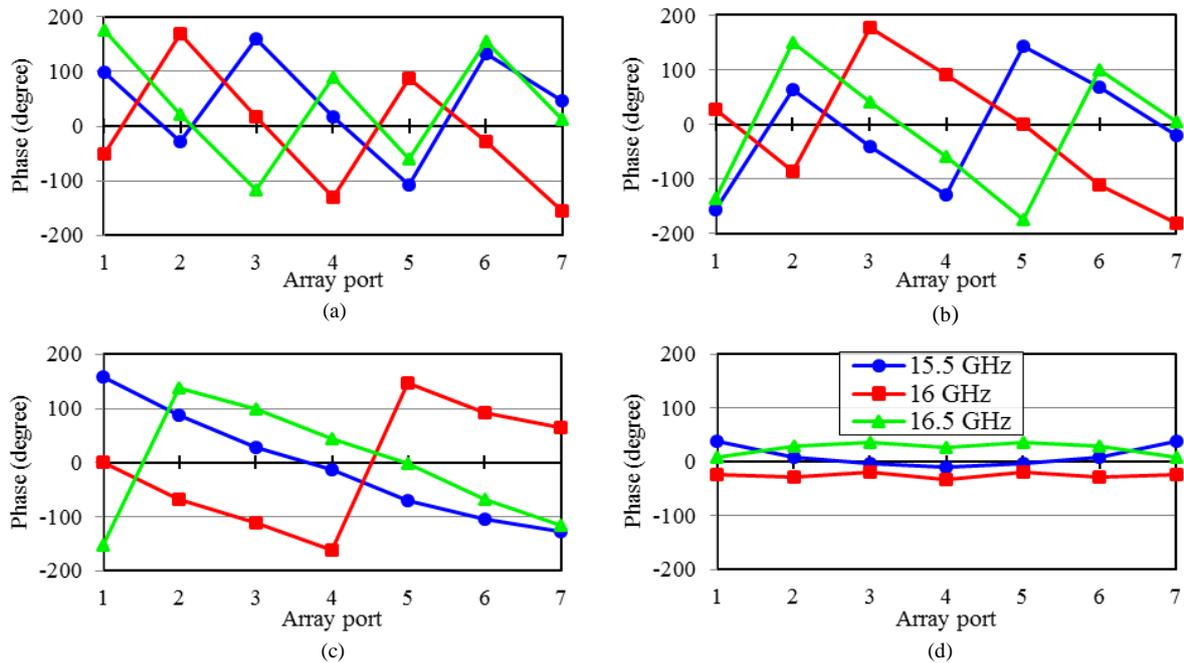
Fig. 7. Array ports relative phase distribution for three frequencies when the beam ports (a) B1, (b) B2, (c) B3 and (d) B4 are excited.
