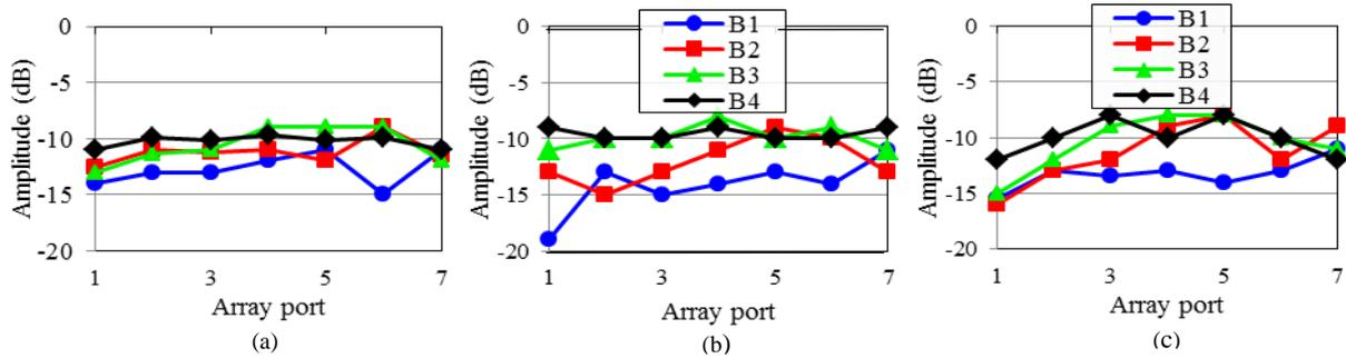
Fig. 6. Array ports amplitude distribution for beam ports B1, B2, B3 and B4 for three frequencies (a) 15.5 GHz, (b) 16 GHz (c) 16.5 GHz.
