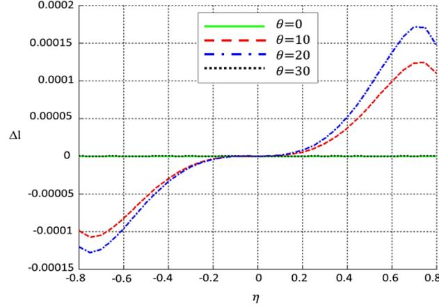
Fig. 4. Normalized path length error of Rotman lens ( $g=1.125$ ,  $\alpha=30$ )
