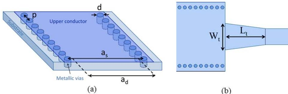
Fig. 3. (a) Structure of the Substrate Integrated Waveguide (SIW). (b) Transition between microstrip line and SIW.
