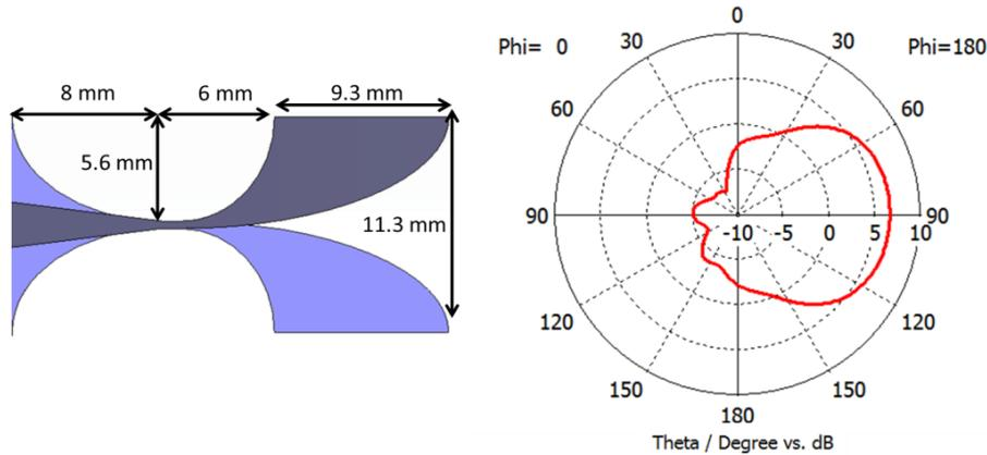
Fig. 8. Vivaldi antenna for 16 GHz and its E-plane pattern.
