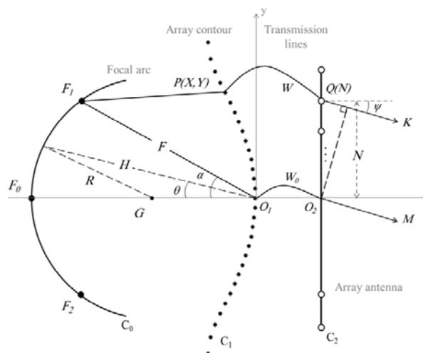
Fig. 2. Parameters of Rotman lens antenna
