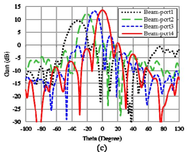
Fig. 10. E-plane radiation patterns of SIW Rotman lens antenna at YOZ plane for (a) 15.5 GHz, (b) 16 GHz and (c) 16.5 GHz. (simulated in CST)
