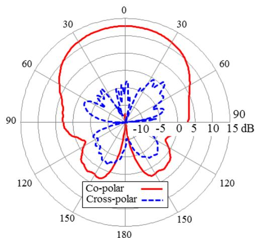
Fig. 12. Co-polar and Cross-polar radiation patterns of beam-port4 of SIW Rotman lens antenna at XOZ plane for 16 GHz. (simulated in CST)
