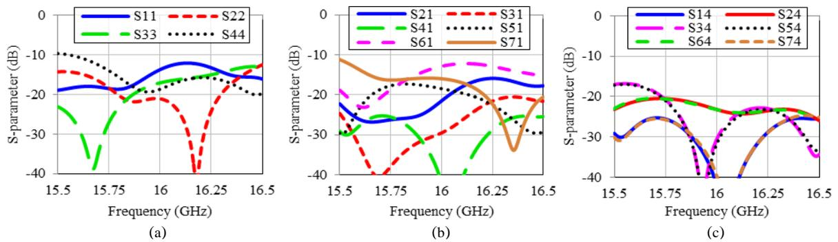
Fig. 9. (a) Reflection coefficients of B1 to B4 beam ports. The coupling between beam ports when (b) B1 and (c) B4 are excited.
