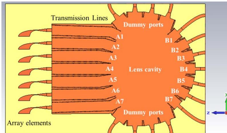
Fig. 5. The modified SIW Rotman lens antenna. The ports that have been named with B and A are the beam ports and array ports respectively.
