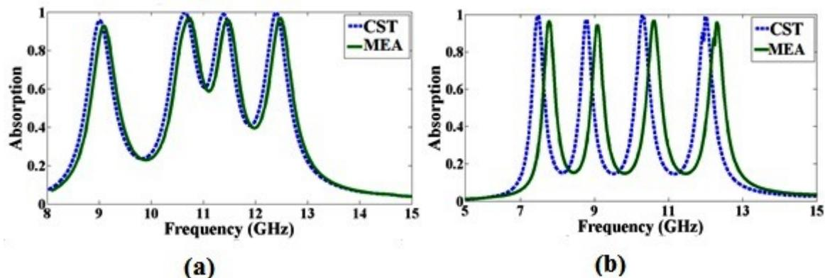
Fig. 7. Simulated (blue curve) and measured (green curve) absorption spectra of the quad-band MA under normal incidence (TM incidence), for the two-layered (a) circular, and (b) square structures.
