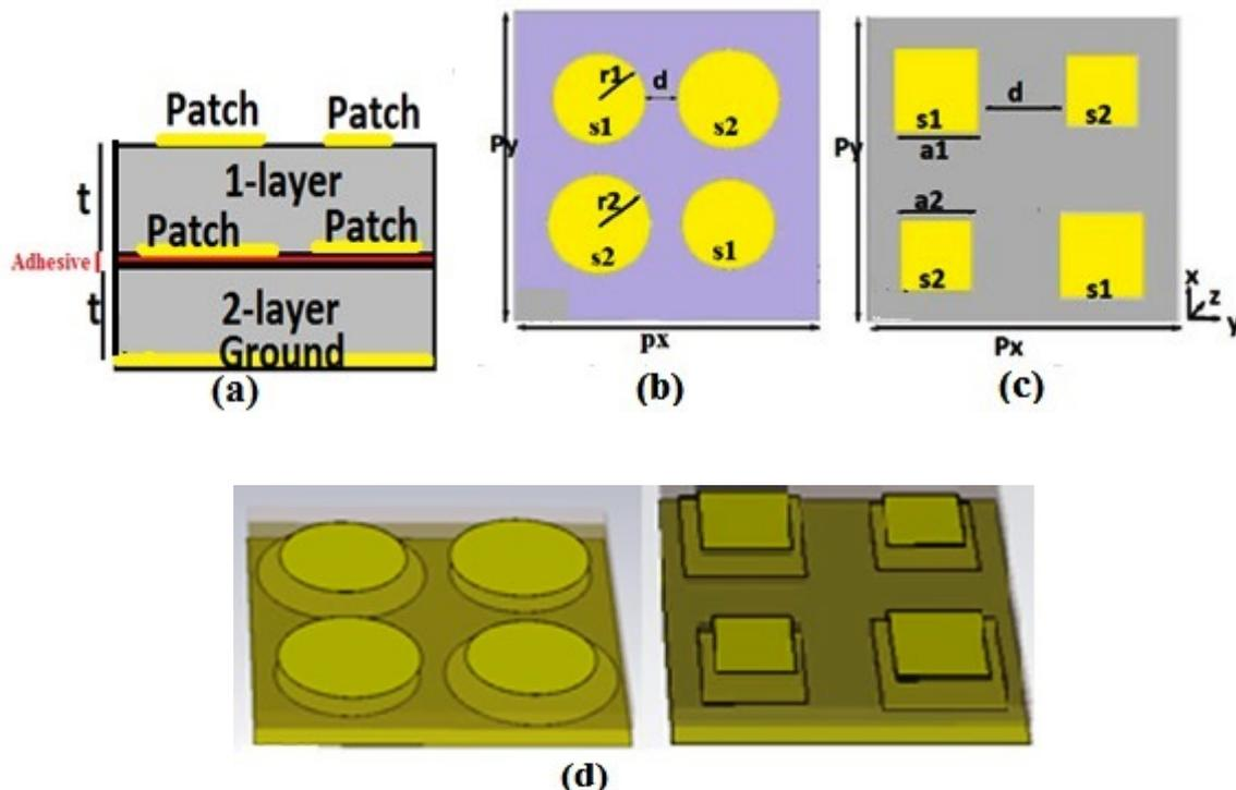
Fig. 1. Perspective view and unit cell geometry of the metamaterial absorbers (a) side view of two-layered structure, (b) top view of circular and (c) top view of square-shaped patches, (d) Simulated MAs samples.
