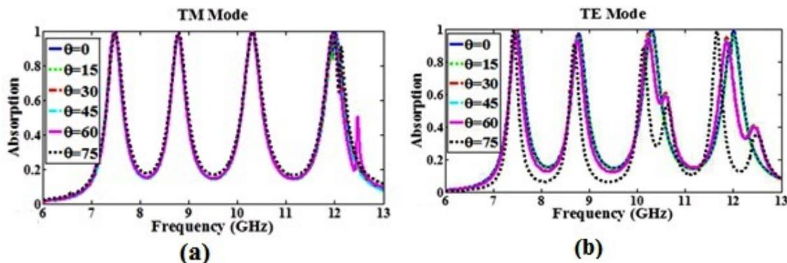
Fig. 3. The simulated results under normal and oblique incidence for two-layered square structure, (a) TM, and (b) TE modes.
