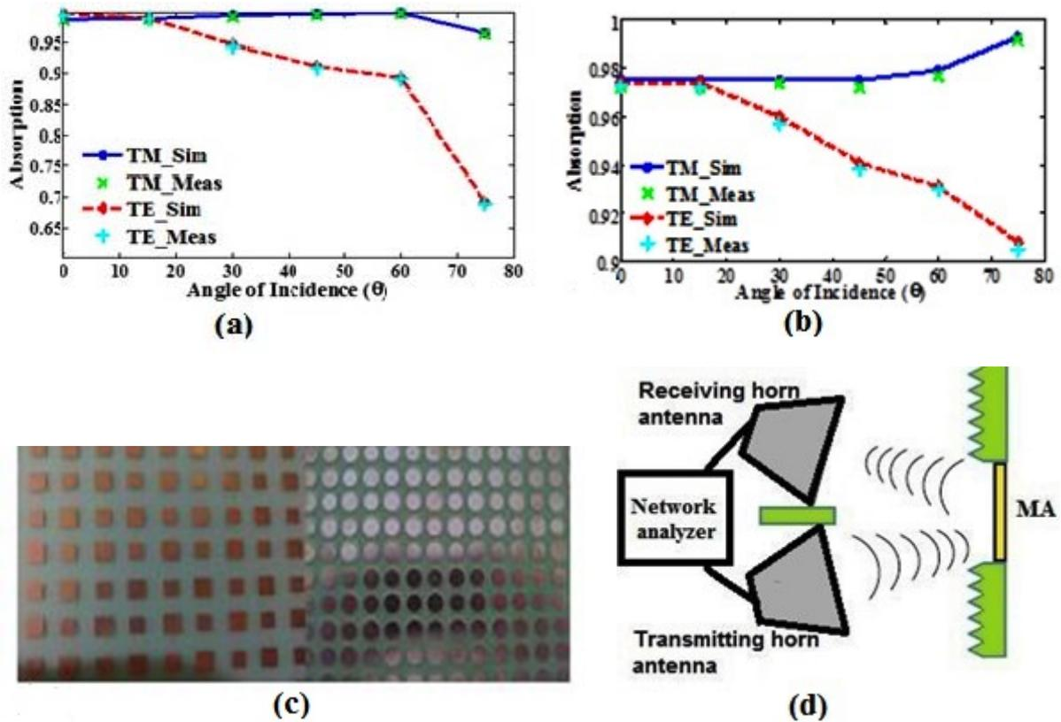
Fig. 6. The comparison of simulated and measured results for the TM and TE modes under normal and oblique incidence, (a) the two-layered structure with circular cells, (b) the two-layered structure with square cells. (c) Fabricated metamaterial absorber, (d) The experimental setup in which the MA sample is placed in the center of flat base.
