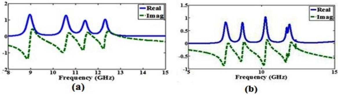
Fig. 4. Retrieved impedance result for two-layered (a) circular, and (b) square structures for TM mode
