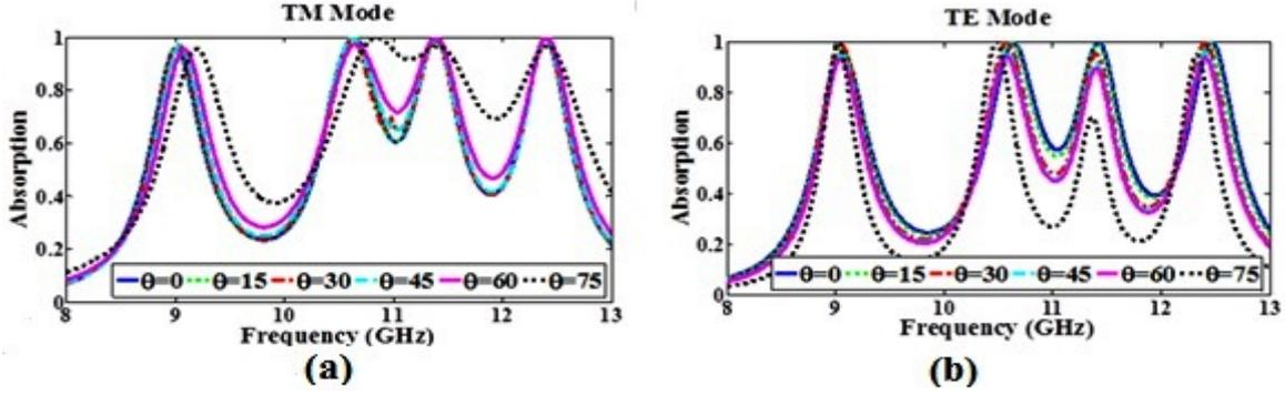
Fig. 2. The simulated results under normal and oblique incidence for two-layered circular structure, (a) TM, and (b) TE modes.
