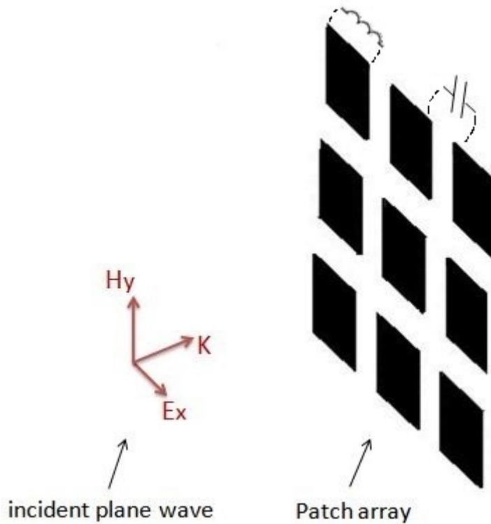
Fig. 4. Describing model for calculating the reactance of patch array.
