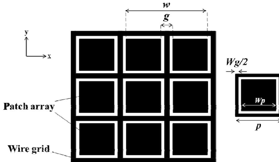
Fig. 1. Geometry of the proposed SRS-FSS and its constituting unit cell.
