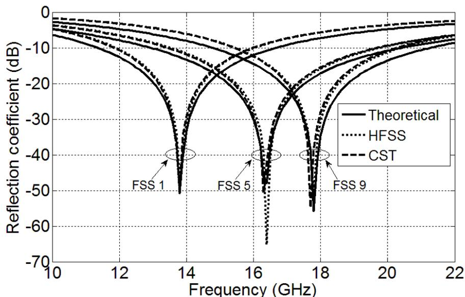
Fig. 7. Reflection coefficients of three different SRS-FSSs for normal incidence.
