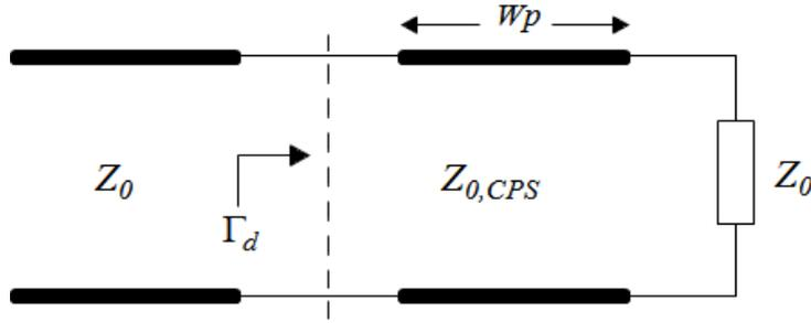
Fig. 6. The proposed model for calculating the coefficient  $R$ .
