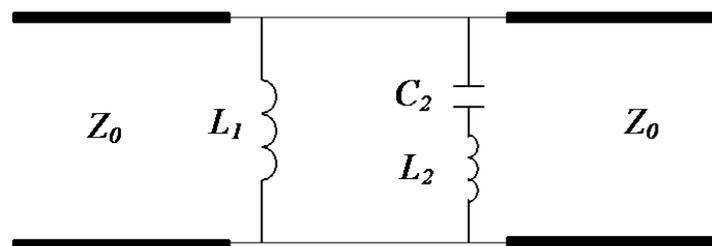
Fig. 2. Equivalent circuit model for the proposed SRS-FSS.
