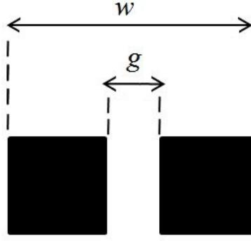
Fig. 5. Geometry of a CPS transmission line comprising two planar strip conductors.
