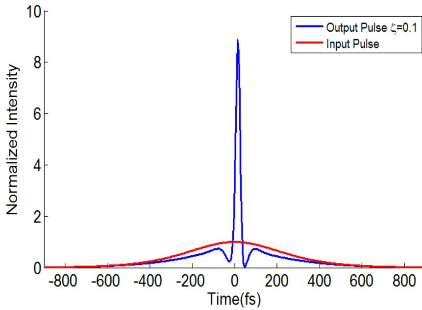
Fig.6. Output compressed pulse at a wavelength of 1550 nm and normalized propagation distance of  $\xi = 0.1$ . Input pulse is also shown.
