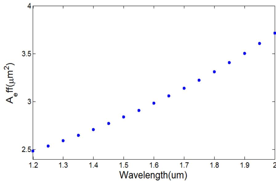
Fig. 5. Effective area of the fundamental mode for the proposed PCF .
