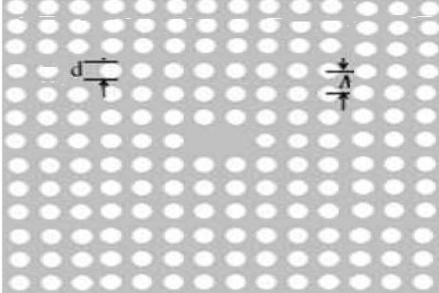
Fig.1. The proposed square lattice PCF schematic.
