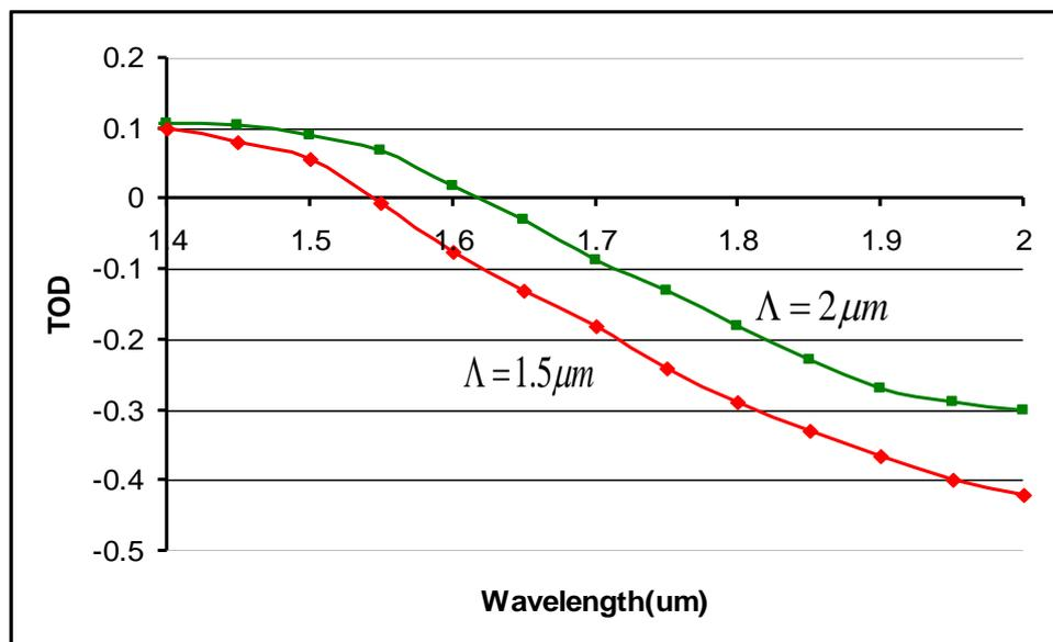
Fig. 4. TOD ( $\text{ps}^3/\text{km}$ ) of the proposed PCF as a function of wavelength for  $\frac{d}{\Lambda} = 0.8$  and several pitches.
