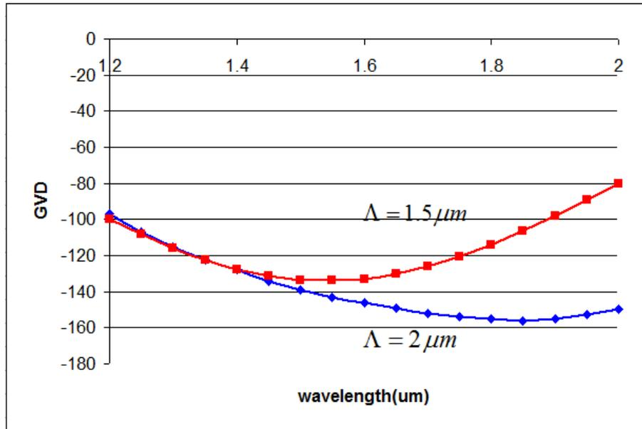
Fig. 2. GVD ( $ps^2/km$ ) of the proposed PCF as a function of wavelength for  $\frac{d}{\Lambda} = 0.8$  and several pitches.
