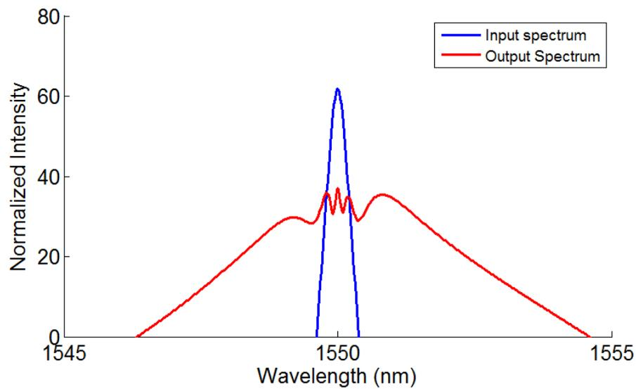
Fig.7. Spectrum of the output compressed pulse at a propagation distance of  $\xi = 0.1$ . The Input Spectrum is also shown.
