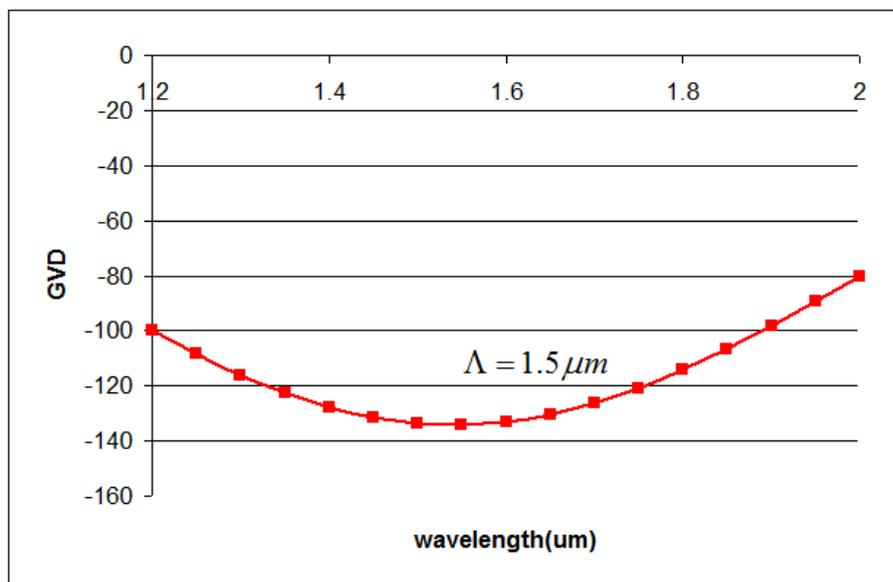
Fig. 3. GVD ( $ps^2/km$ ) of the proposed PCF as a function of wavelength for  $\frac{d}{\Lambda} = 0.8$  and  $\Lambda = 1.5 \mu m$ .
