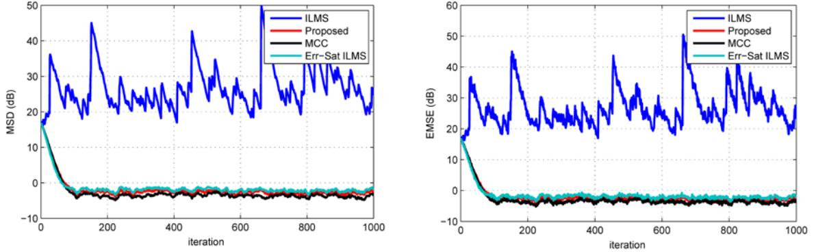
Fig. 4. The global average MSD and global average EMSE for different algorithms in the presence of impulsive noise.
