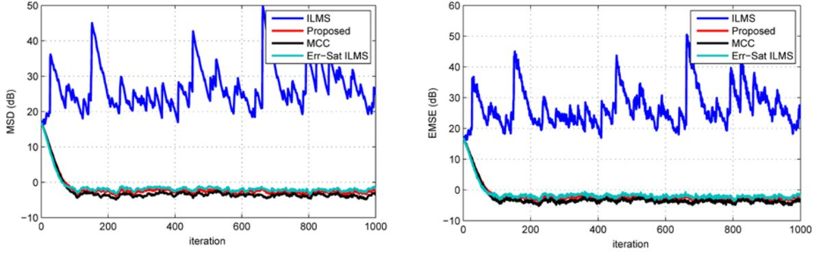
Fig. 4. The global average MSD and global average EMSE for different algorithms in the presence of impulsive noise.
