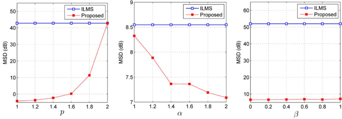
Fig. 5. Performance of the proposed algorithm for different values of noise parameters in comparison with the ILMS algorithm.
