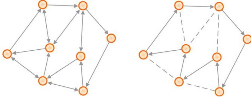
Fig. 1. Different cooperation modes for adaptive networks: Incremental (left) and diffusion (right).
