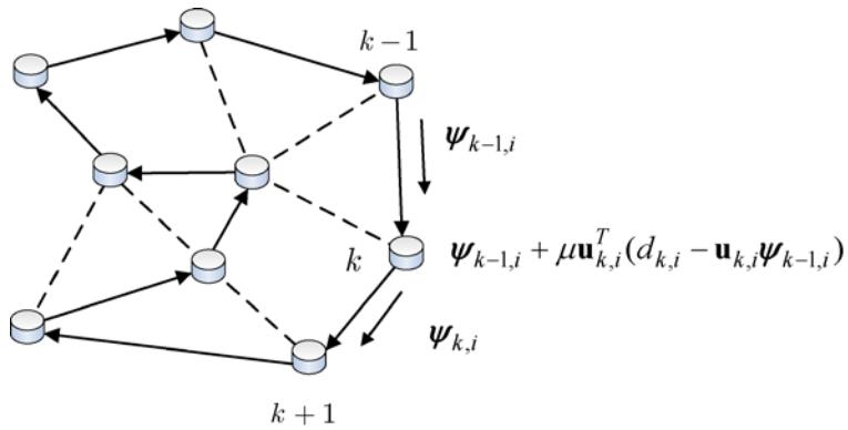
Fig. 2. The structure of incremental LMS algorithm.
