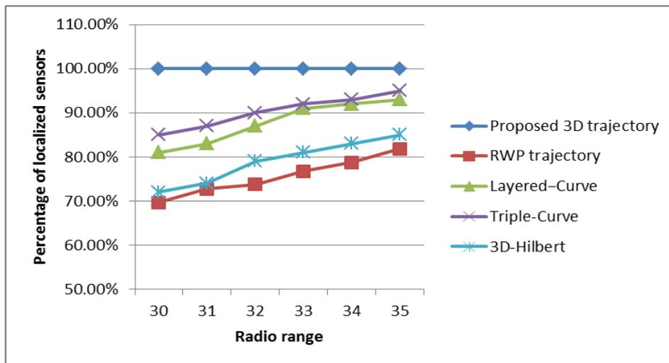
Fig. 10. Radio range versus percentage of positioned sensor nodes.
