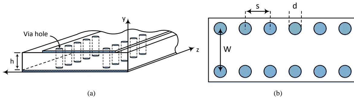
Fig. 1. Configuration of the SIW structure (a) solid view (b) top view.
