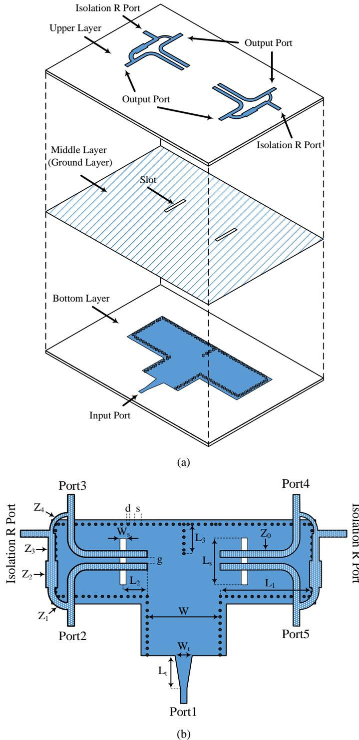
Fig. 2. Configuration of the proposed structure (a) solid view (b) top view.
