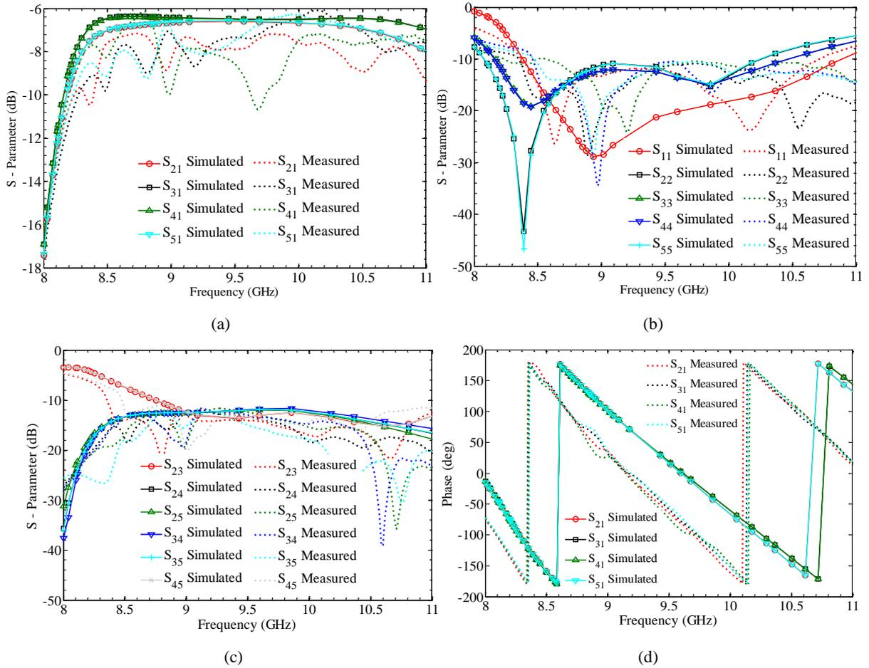
Fig. 6. Simulated and measured (a) insertion loss (b) return loss (c) isolation between output ports (d) phase.
