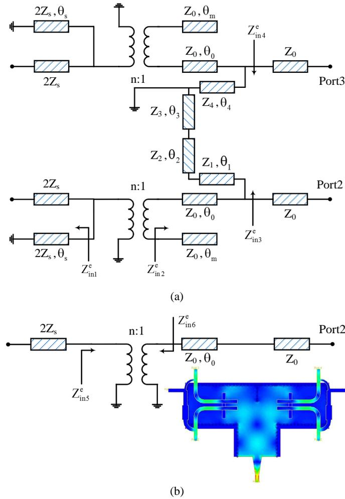
Fig. 3. (a) Even-mode equivalent circuit and (b) simplified even-mode equivalent circuit of the proposed SIW power divider.
