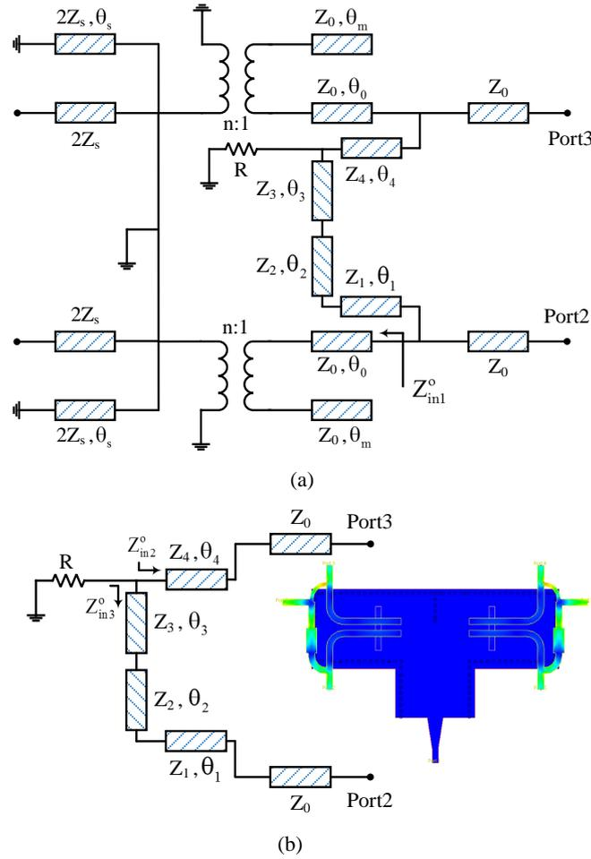
Fig. 4. (a) Odd-mode equivalent circuit and (b) simplified odd-mode equivalent circuit of the proposed SIW power divider.
