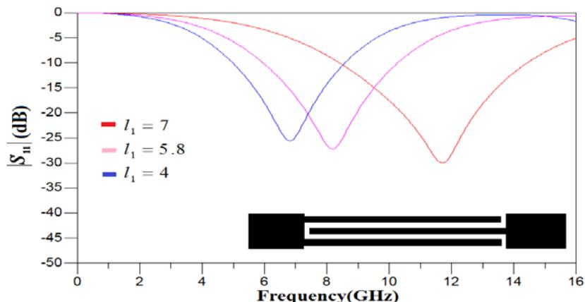
Fig. 4. Frequency response ( $|S_{12}|$ ) of the microstrip ring with doublets parallel coupling gaps when the length  $l_1$  of the parallel coupling gaps is 4mm, 5.8mm, and 7mm, respectively.
