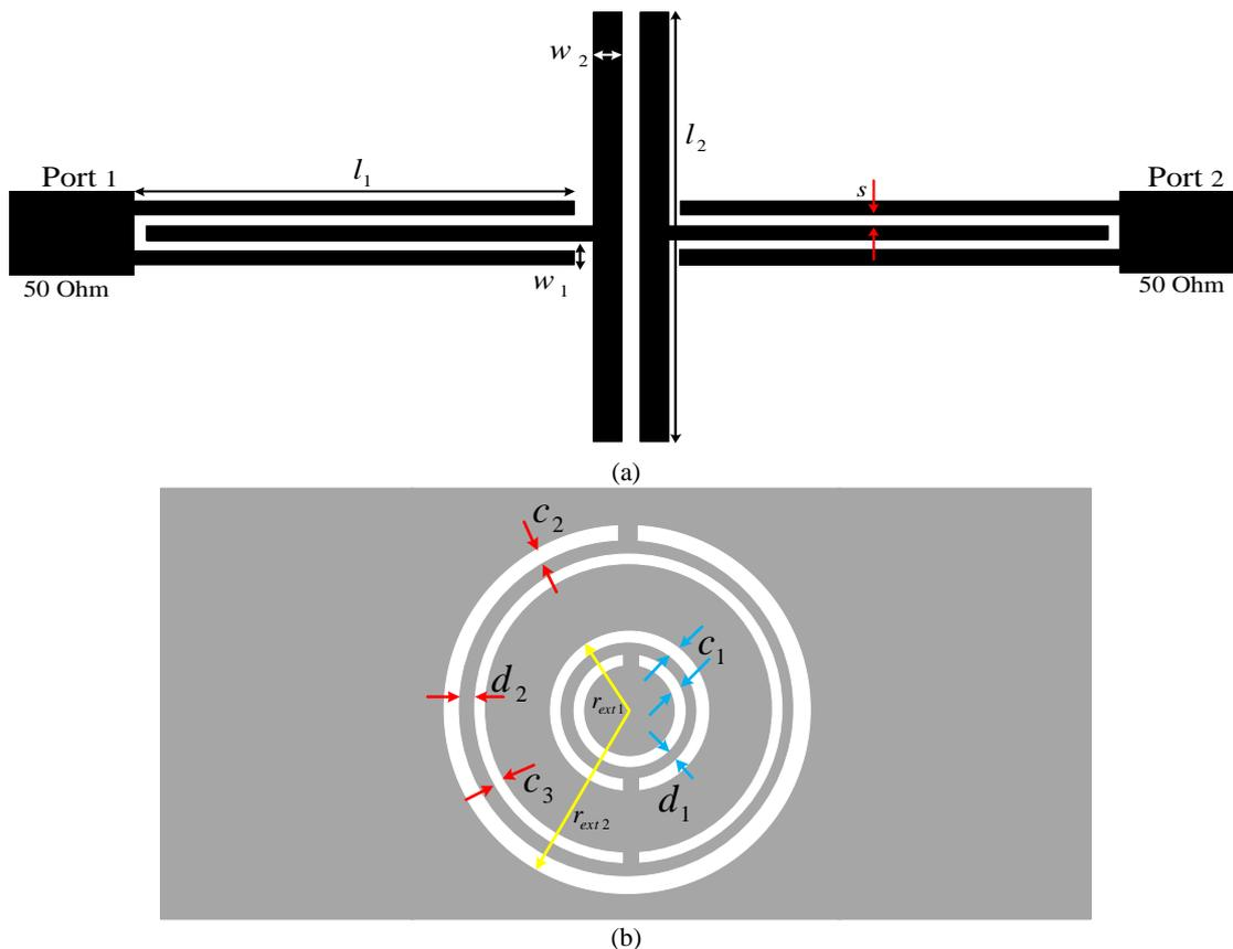
Fig. 3. Configurations of the proposed UWB filter. (a) Top and (b) bottom layers.
