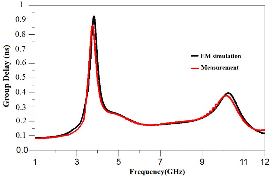
Fig. 8. Simulated and measurement Group delay of the proposed UWB Filter.
