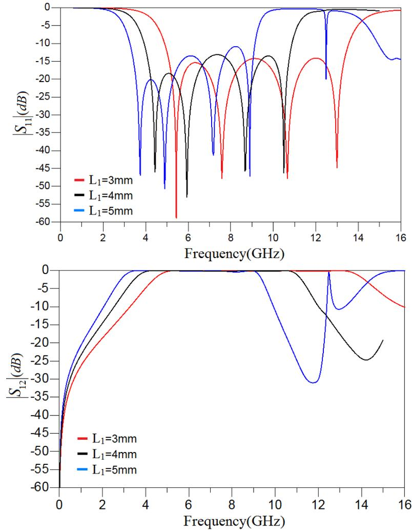
Fig. 5: Frequency response ( $|S_{11}|$  and  $|S_{12}|$ ) of the microstrip series capacitor with doublets parallel coupling gaps when the length  $l_1$  of the parallel coupling gaps is 3mm, 4mm, and 5mm, respectively. Other dimensions are:  $w_1 = 2.8$  mm,  $l_2 = 4$  mm,  $w_2 = 0.6$  mm.
