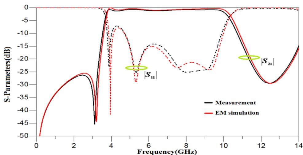
Fig. 7. Simulated and Measured frequency responses of the proposed UWB Filter.
