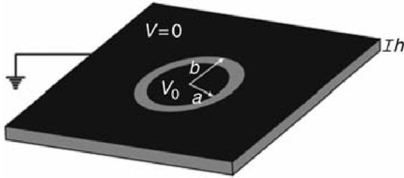
Fig. 2. The capacitance and inductance of the CSRR is approximately equal to that corresponding to a metallic disk of radius  $a = r_0 - c/2$  surrounded by a ground plane at a distance  $b - a = c$ ,  $r_0$  is the averaged radius of the CSRR and  $c$  is the width of the slots. The dielectric substrate is characterized by its permittivity  $\epsilon$  and thickness  $h$  [21].
