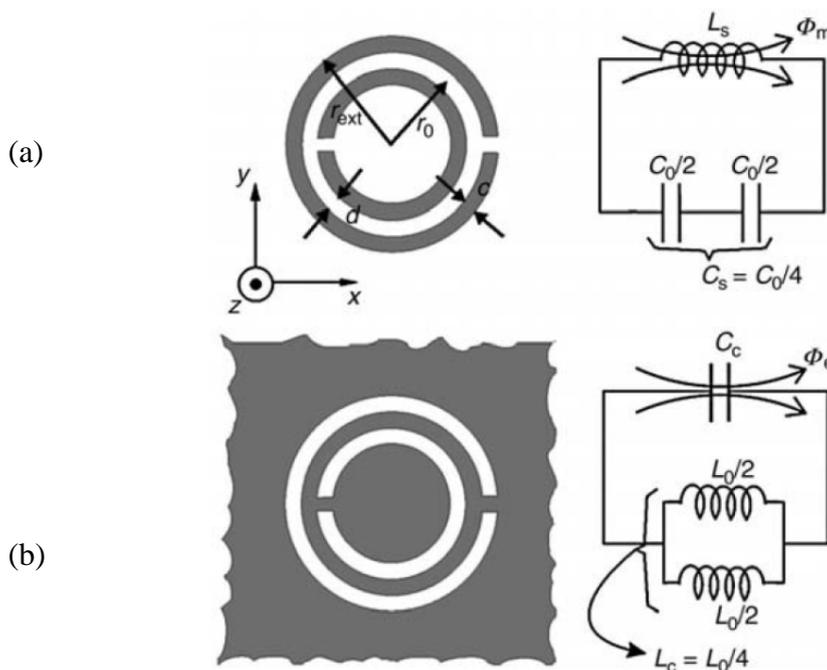
Fig. 1. Topologies of (a) the SRR and (b) CSRR, and their equivalent circuit models [21].
