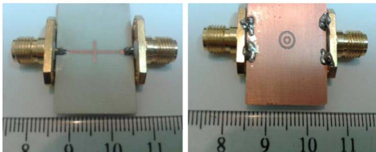
Fig. 6. Top and bottom views of the fabricated UWB filter.
