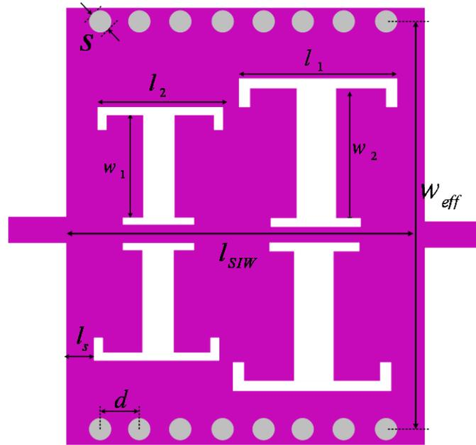
Fig. 1. Configurations of the proposed SIW T-shape slot filter.
