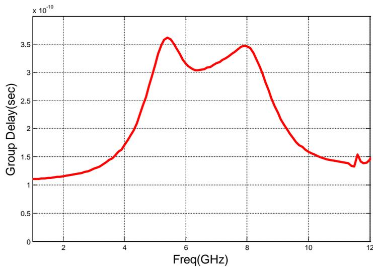
Fig.9. Simulated group delay of the proposed filter.
