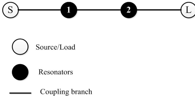
Fig. 2. Coupling topology of a proposed SIW filter with two poles.
