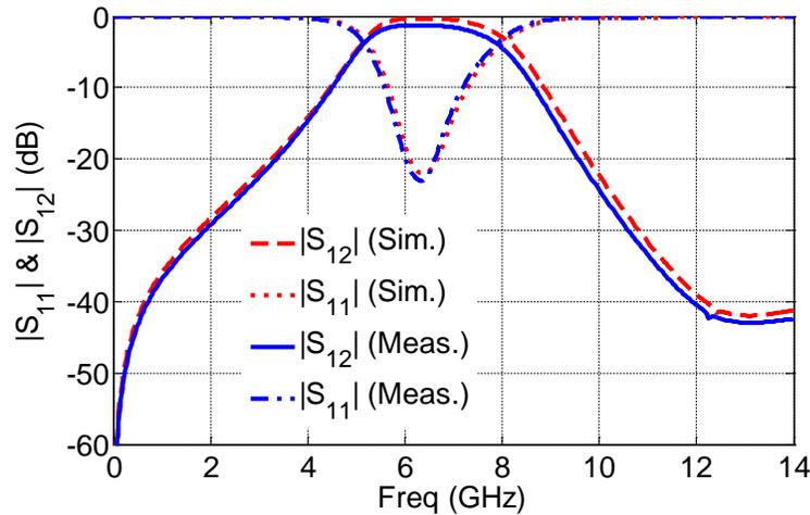
Fig. 7. Simulated and measured frequency responses of the proposed wideband filter.
