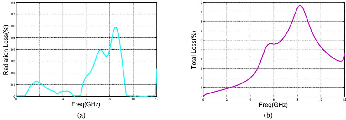
Fig.8. (a) The simulated radiation loss and (b) The simulated total losses of the proposed filter.
