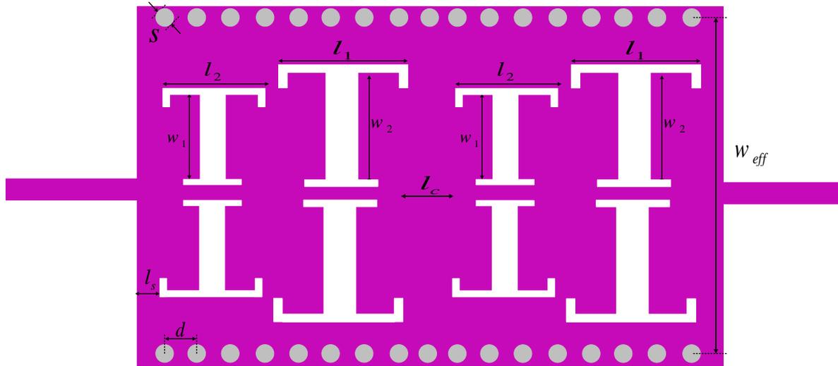
Fig.5. Configuration of the proposed two-stage SIW filter with its geometric parameters listed in Table II.
