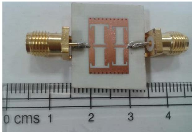
Fig.10. Photograph of the fabricated filter.
