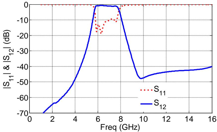
Fig.6. Simulated results for the SIW filter loaded by two-cells of the T-shaped resonators.
