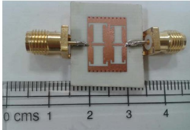
Fig.10. Photograph of the fabricated filter.
