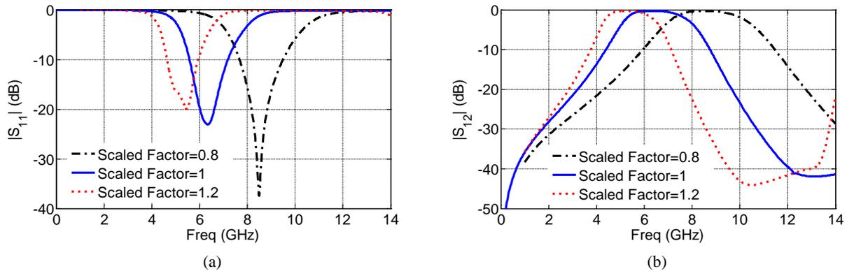
Fig.4. Frequency responses (a)  $|S_{11}|$  and (b)  $|S_{12}|$  of the proposed SIW filter when the whole dimensions, multiple in variation factor.
