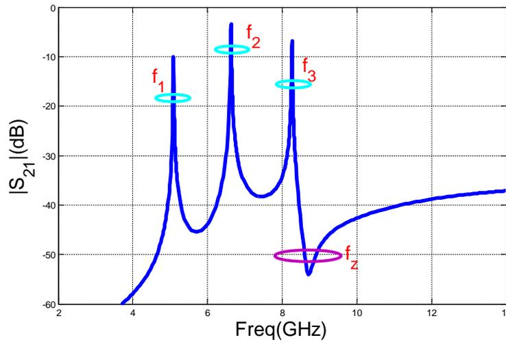
Fig.3. Simulated frequency responses of the proposed filter with weak coupling.
