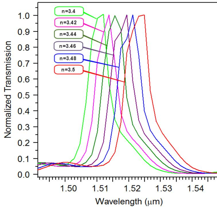
Fig. 6. Normalized power transmission spectra of the proposed CDF for different values of refractive index of dielectric rods.
