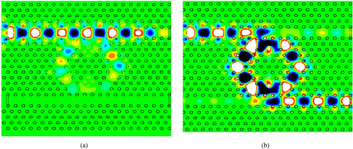
Fig. 5. Electric field pattern of the ring resonator at (a) 1501.4 nm (non-resonant wavelength) and (b) 1519.4 nm (resonant wavelength).
