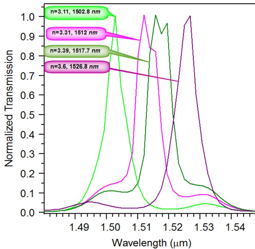
Fig. 7. Normalized power transmission spectra of the proposed CDF for different values of refractive index of inner rods
