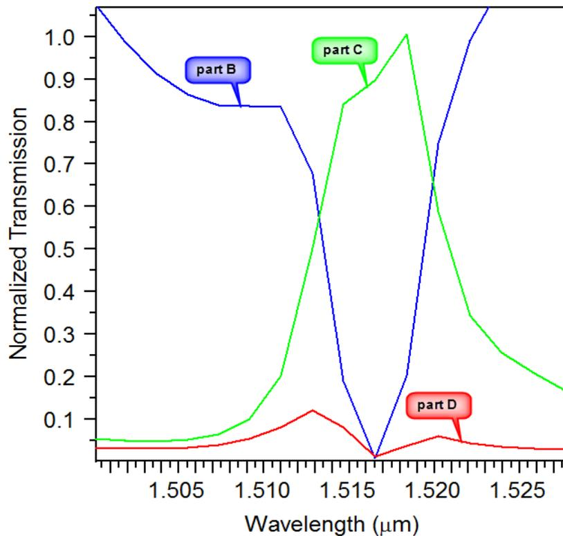
Fig. 4. Transmission spectra of the CDF at ports B, C and D respectively.
