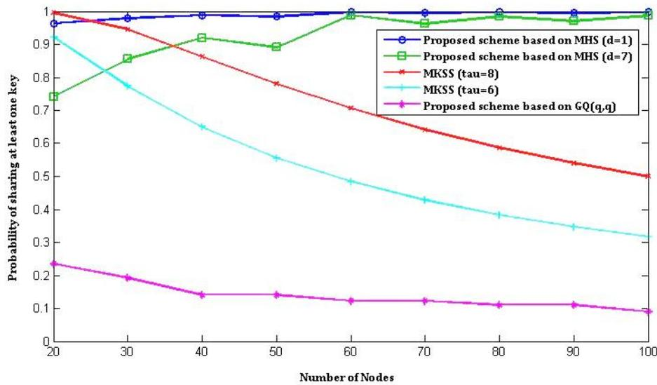
Fig. 1 Probability of sharing at least one key (connectivity) when two nodes each randomly chooses  $\tau$  spaces from  $\omega$  spaces in the MKSS and the proposed scheme based on combinatorial properties of various combinatorial frameworks for parameters  $\omega$  and  $\tau$ .
