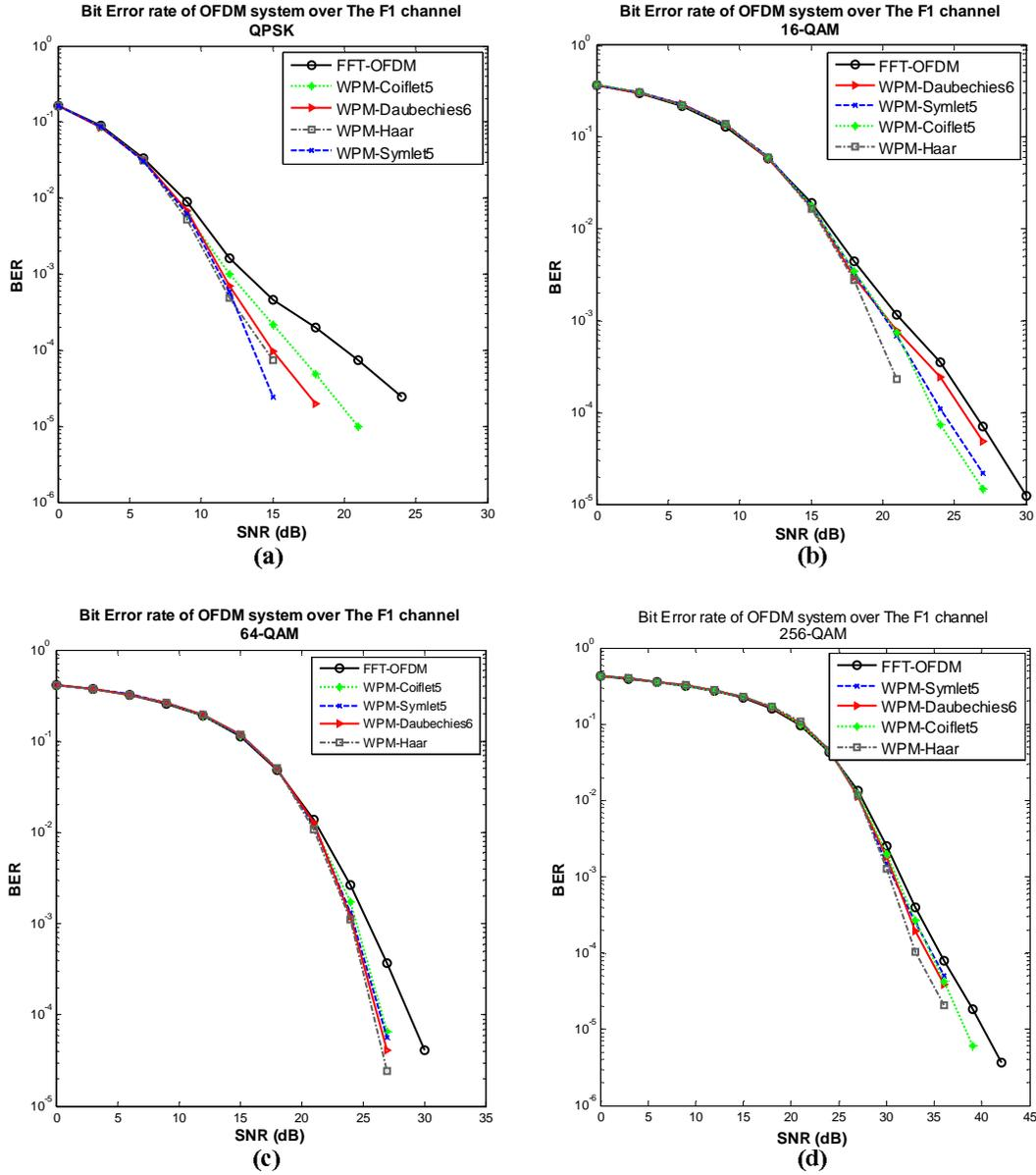
Fig. 9. BER of FFT-OFDM and WPM for F1 channel with (a) QPSK, (b) 16-QAM, (c) 64-QAM and (d) 256-QAM
