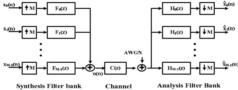
Fig. 1. Block diagram of filter bank-based MCM system
