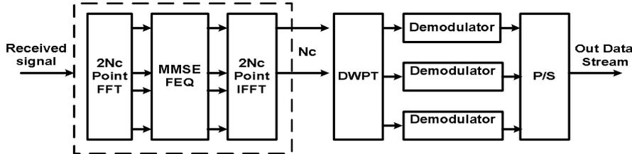
Fig . 5. The structure of overlap FEQ equalizer
