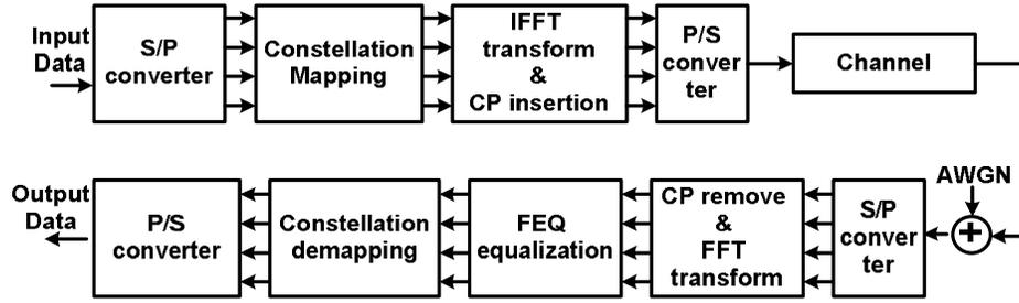
Fig. 2. Transceiver structure of FFT-OFDM system
