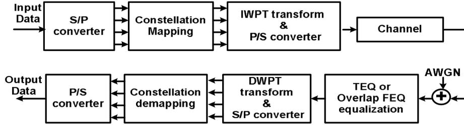
Fig. 3. Transceiver structure of WPT-OFDM system
