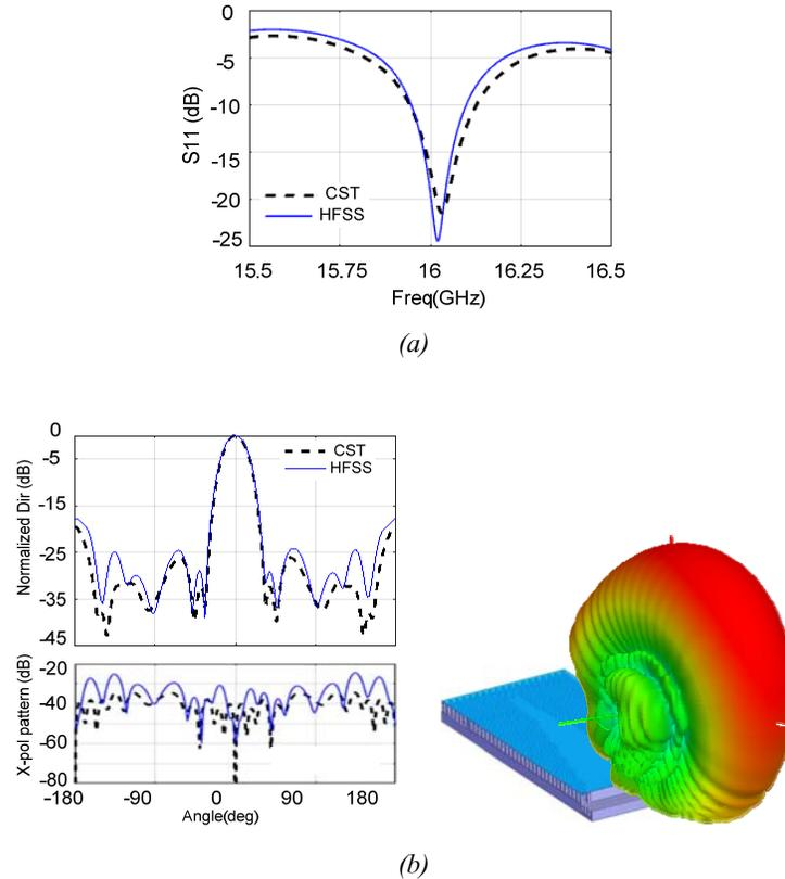
Fig. 5. Simulation results (CST & HFSS) for the back lobe suppressed GGW H-plane horn presented in Fig. 1(b).
