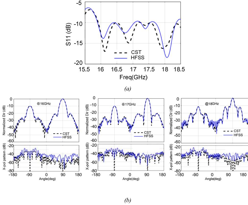
Fig. 4. Simulation results (HFSS & CST) for the ordinary GGW H-plane horn presented in Fig. 1(a). (a) Reflection coefficient ( $S_{11}$ ) and (b) Radiation patterns at H-plane (co- & cross) at three frequencies over the whole bandwidth.
