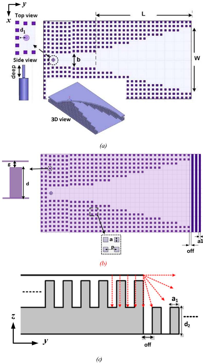
Fig. 1. The structure of proposed GGW H-plane horn antenna. (a) without any back lobe suppression Mechanism, (b) Using corrugations as a back lobe suppression mechanism (top view) and (c) Side view of Fig. 1(b).
