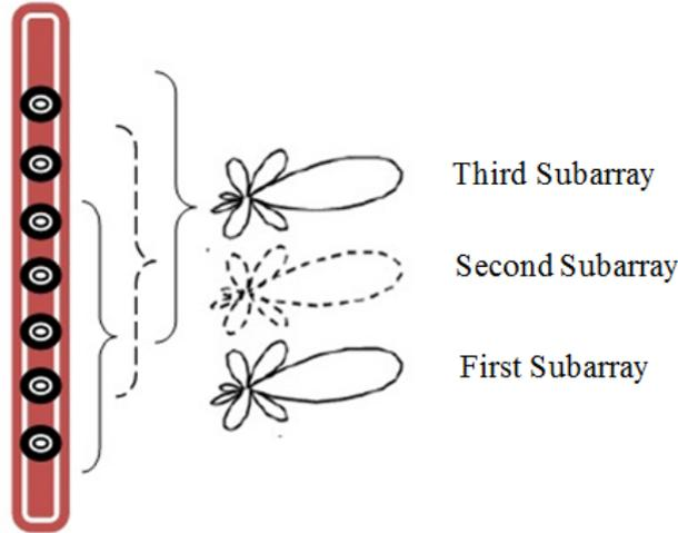
Fig. 1. A phased-MIMO radar with 3 subarrays.
