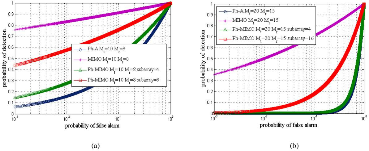
Fig. 2. Comparison of receiver-operating-characteristic (ROC) curves in GLRT detectors with (a)  $M_t=10, M_r=8$ , and (b)  $M_t=20, M_r=15$
