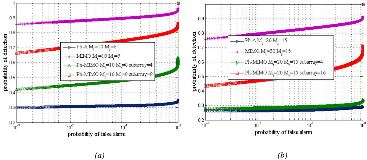
Fig. 3. Comparison of receiver-operating-characteristic (ROC) curves in LRT detector with (a)  $M_t=10$ ,  $M_r=8$ , and (b)  $M_t=20$ ,  $M_r=15$
