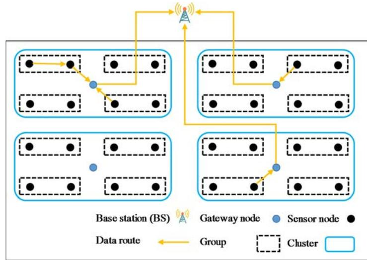
Fig. 4. A network model of the new proposed algorithm.
