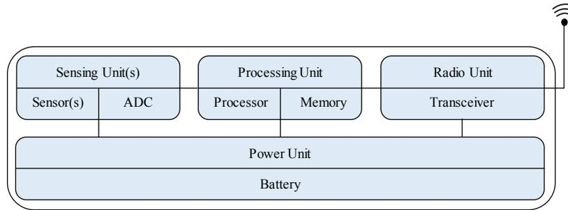
Fig. 1. Common sensor node units.
