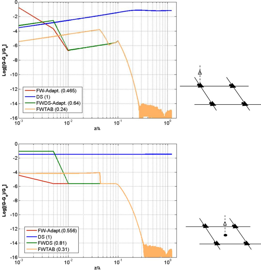
Fig. 4. Comparison of methods in terms of accuracy and computation time (normalized to that of DS): An array with  $s_x = s_y = 0$  is assumed and period of  $X = Y = 1.2$  wavelength. the DS results are obtained by taking  $200 \times 200$  point sources into account. Points above  $(x = y = 0)$  (top) and above  $(x = 0.5X, y = 0.5Y)$  (bottom).
