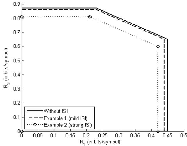
Fig. 4 Capacity inner bounds of the channels in examples 1 and 2 as well as of the channel without ISI.
