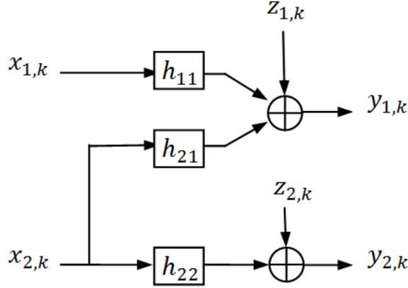
Fig. 2 The discrete-time linear Gaussian ZC with ISI.
