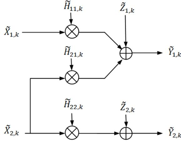
Fig. 3 The  $k$ th-component channel.
