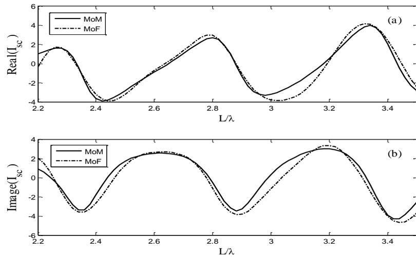
Fig. 14. Predicted lightning induced current for  $X_s = 50m$  and comparing with MoM.
