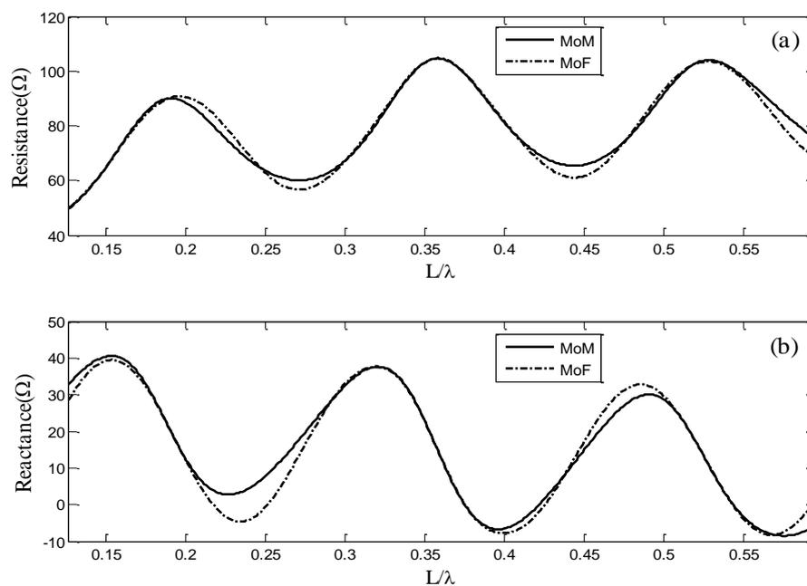
Fig. 17. Comparing the modelled input impedance by MoM and MoF.
