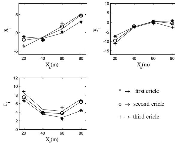
Fig. 13. Centre coordinates and radius of three fitted circles versus  $X_s$  in meter as the fitted curves of second-order.
