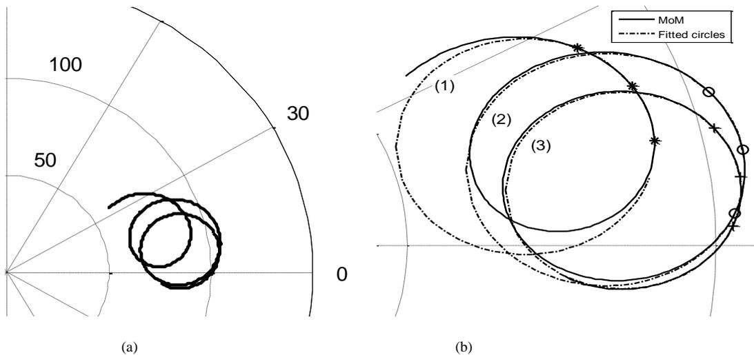
Fig. 15. (a) Amplitude versus phase of the input impedance (ohm) of buried rod inside soil, (b) figure (a) in zoomed form in addition to starting points (stars, circles, and pluses) and fitted circles (dash-dotted).
