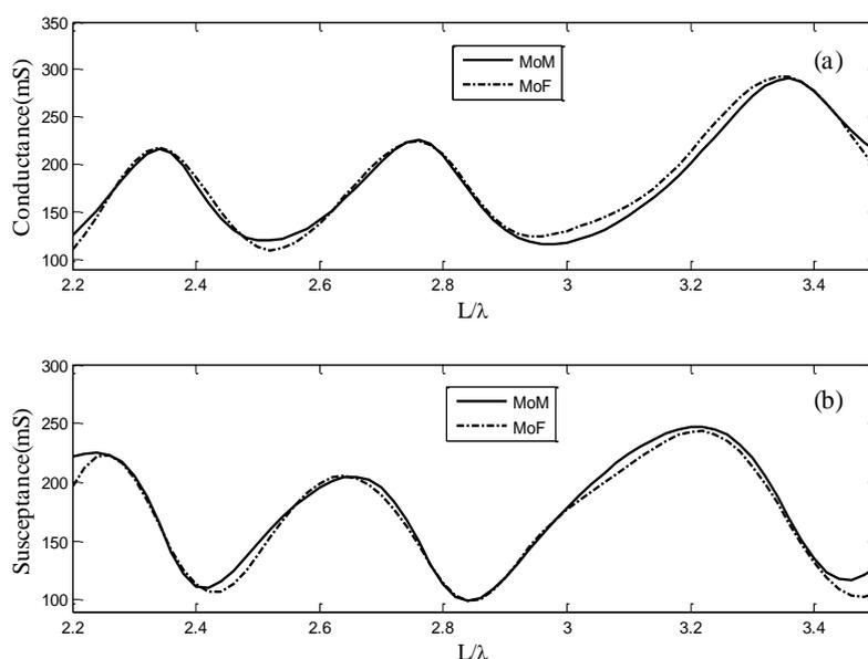
Fig. 9. Output Comparing the modeled input admittance with the MoM. (a) Real part. (b) Imaginary part.
