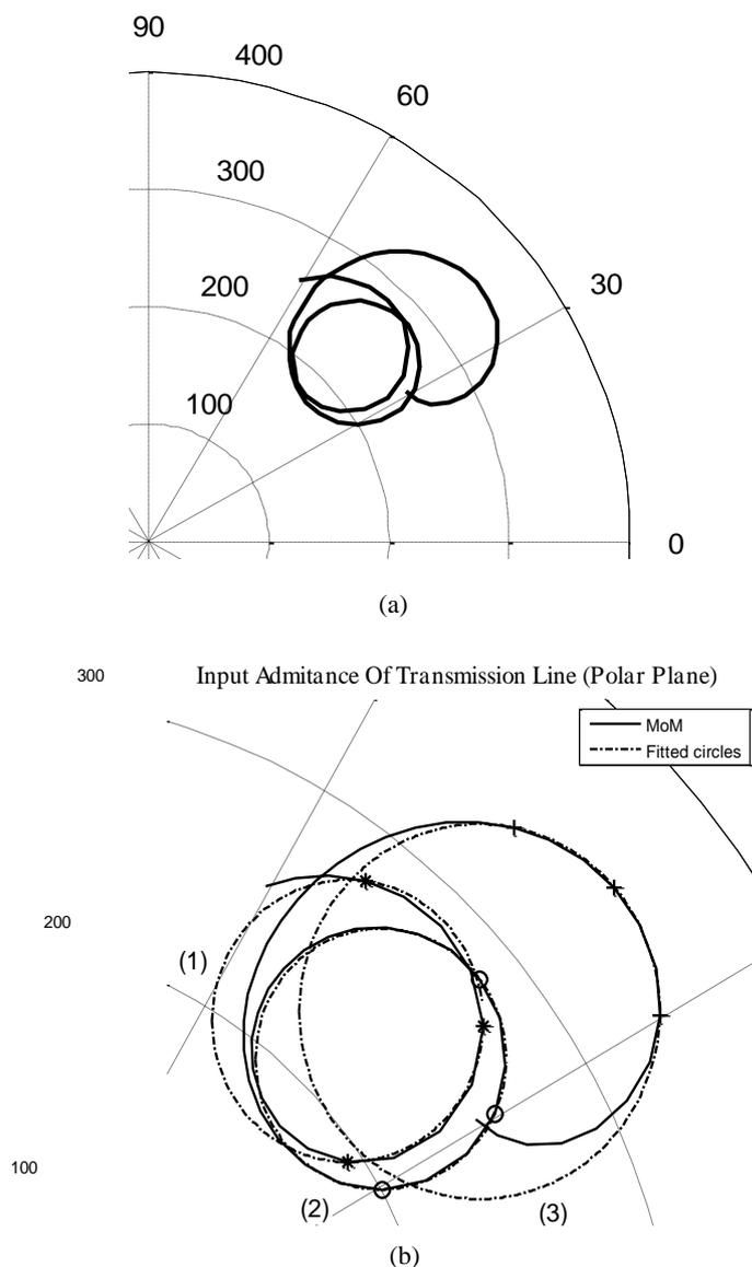
Fig. 4. (a): Amplitude versus phase of the input admittance in polar plane by MoM (b) figure (a) in zoomed form in addition to starting points (stars, circles and pluses) for defining fitted circles.
