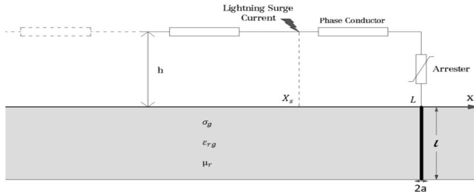
Fig.1. Schematic diagram of a single-conductor transmission line above a lossy ground with a grounded lightning arrester.
