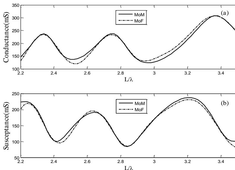
Fig. 11. Predicted input admittance of the overhead line compared with the MoM for  $h = 19m$ .
