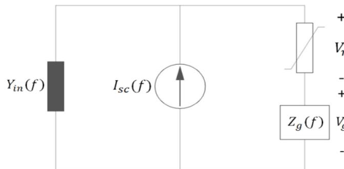
Fig. 3.Equivalent circuit model of the problem shown in figure 1 (a) and (b) ignoring the ionization of soil.
