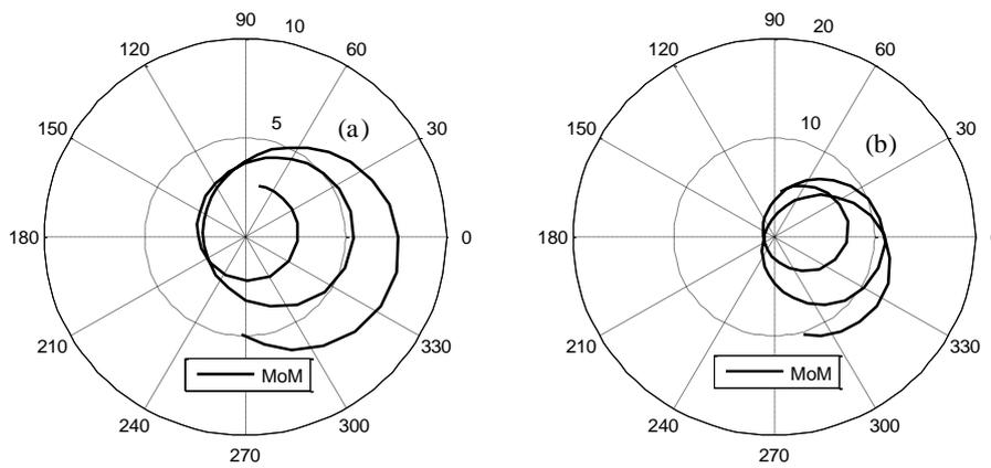
Fig. 12. Short circuit current in polar plane. (a)  $X_s = 60m$  . (b)  $X_s = 80m$  .
