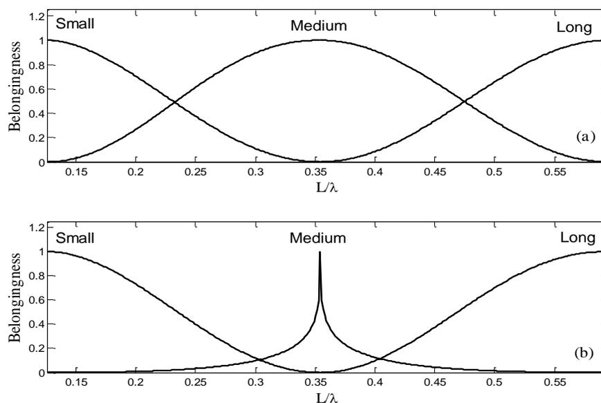
Fig. 16. The optimized membership functions for modelling (a) partial locus, (b) partial phase.
