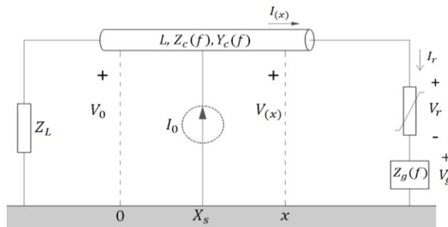
Fig.2.Representation of problem of figure 1(a) by transmission line model.
