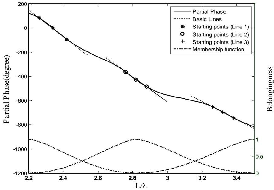
Fig. 7. partial phase, fitted line and membership functions for modeling partial phase.
