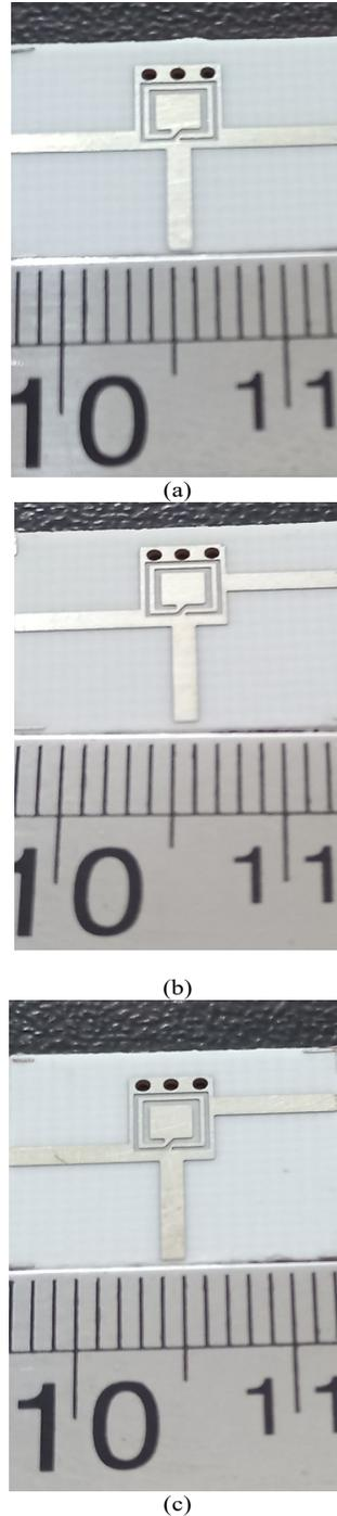
**Fig. 15. Photograph of the fabricated equal/unequal HMSIW-CSR FPDs:
