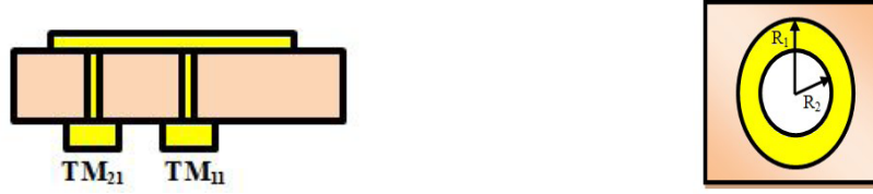
Fig. 5. Geometry of the element antenna (a) side view (b) top view
