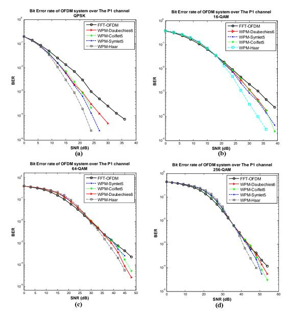
Fig. 8. BER of FFT-OFDM and WPM in P1 channel with (a) QPSK (b) 16-QAM (c) 64-QAM (d) 256-QAM
