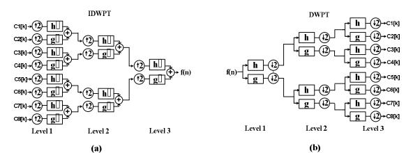
Fig. 4. The structure of (a) WPT synthesis filter bank used in the transmitter (b) WPT analysis filter bank used in the receiver
