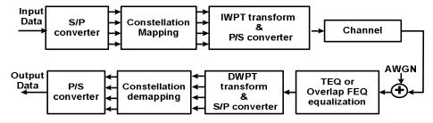
Fig. 3. Transceiver structure of WPT-OFDM system
