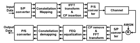
Fig. 2. Transceiver structure of FFT-OFDM system
