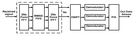
Fig. 5. The structure of overlap FEQ equalizer
